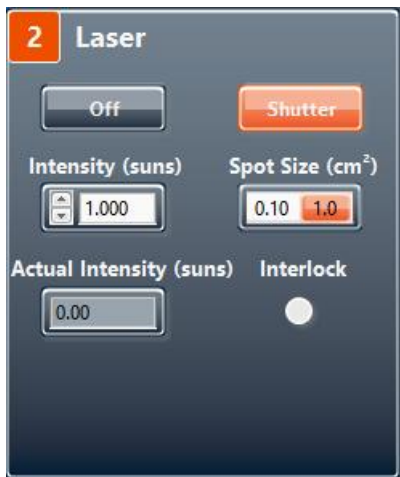
Figure 7: revised section 2 'Laser' with changed button arrangement and new spot size slider.
