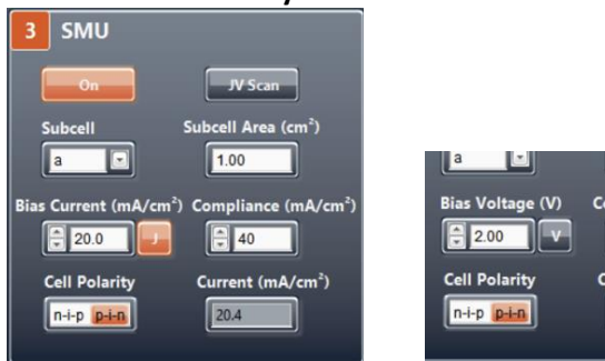
Figure 5: revised section 3 ‘SMU’ with added current density control mode left and traditional voltage control mode right. The modes can be changed by clicking the ‘J’ or ‘V’ buttons..
