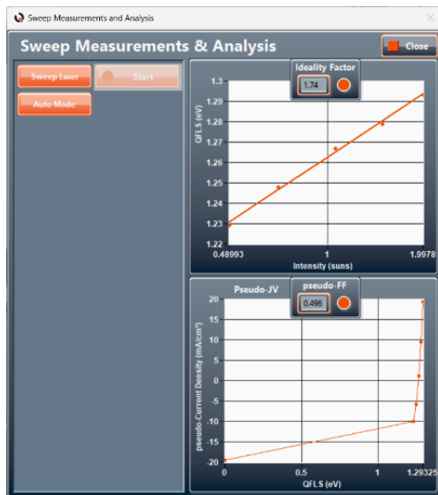
Figure 3: new automated measurement sweep with ideality factor and pseudo-JV extraction.
