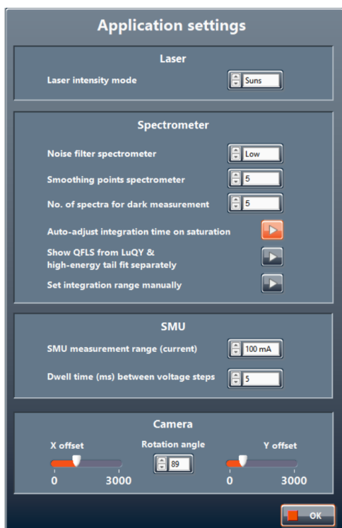
Figure 9: revised application settings window with new functions to show QFLS prediction from LuQY and high-energy tail fit method as well as to set the wavelength range for photon flux integration in LuQY calculation manually.
