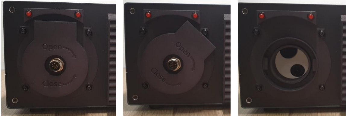
Fig. 4-4. Sample port front view with closed sample holder (left), 45° tilted sample holder (middle) and opened sample port (right)
